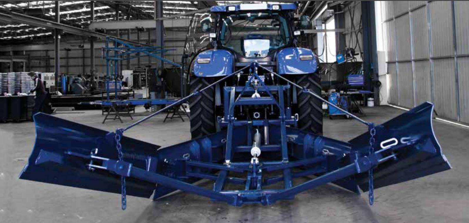
The proven performance of our second generation Channeller provides irrigation farmers an efficient way to clean and construct irrigation channels.
